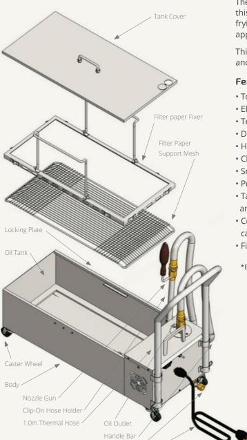
The Fryrite Filter Machine purifies down to 12 microns this means a dramatic extension of the life and quality of frying oil. This will save you the cost of the machine within approximately 6 months!\*
